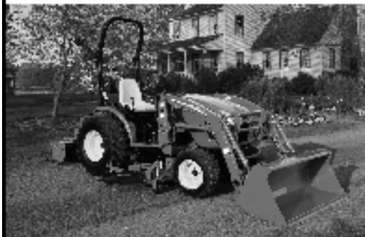
John Deere 2520 Compact Utility Tractor with front loader and rear PTO shaft
